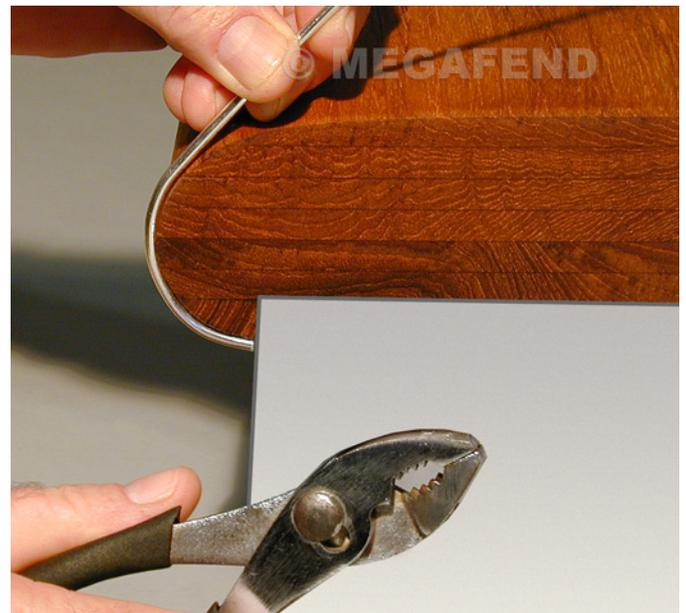
**Step 4—** Continue following contour using pliers as aid in bending rod to assure snug fit.
